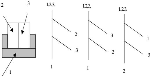
Fig. 5. Disassembly trees
